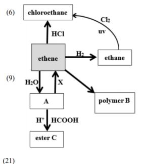
(d) Ester C is formed when A is heated with methanoic acid and a few drops of sulfuric acid acting as a catalyst.
